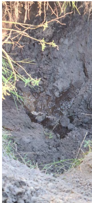
PHOTOGRAPH 4 Test pit TP6, thin layer of fill, with sand directly beneath, with groundwater seepage.
